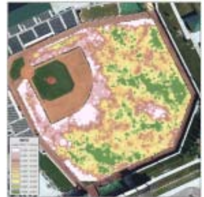
Typical map rendered via GIS software from data collected and georeferenced utilizing ACS-210 Crop Circle Sensor
